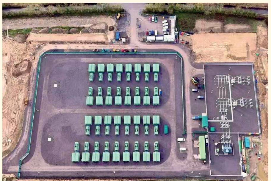
PowerTitan 2.0 can be installed back-to-back with a distance of 15 cm and with no loss of performance.
