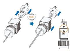
step 5 Fit the seal and the cable gland.
