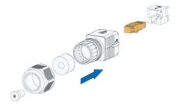
step 2 Tighten the connector housing assembly at the specified torque.
