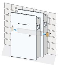
**step 4** Secure brackets a and b together using screws. Then, secure bracket c on the other side of bracket b in the same way.
