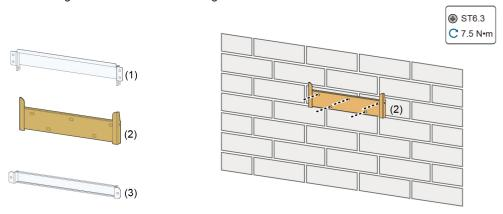
**step 6** Hang the battery onto the mounting bracket on the wall from top to bottom. Ensure that mounting brackets 1 and 2 align properly and tightly against each other, then secure them together with M6 screws.
