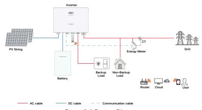
figure 2-1 System Diagram
