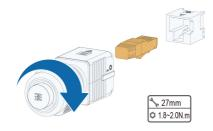
step 3 Attach the matching resistor to the adapter.
