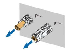
step 2 Insert the connectors into P1+ and P1- terminals, and make sure they "click" into place.
