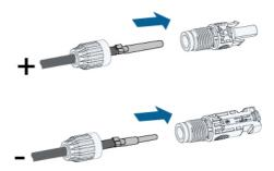
step 4 Tighten the cable gland and the insulator.
