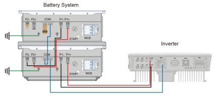
figure 5-4 Front-to-Back Battery Arrangement
