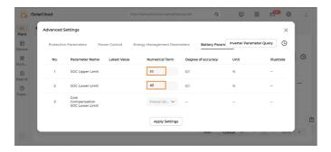
3. Select Charge as the charging command and an appropriate charging power. Monitor the charging process to ensure the SOC reaches 40%. Once charging is complete, disconnect the battery from the hybrid inverter safely.
