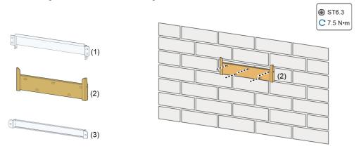
**step 5** Hang the battery onto the mounting bracket on the wall from top to bottom. Ensure that mounting brackets 1 and 2 align properly and tightly against each other, then secure them together with M6 screws.
