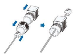
**step 4** Attach the adapter to the RJ45 plug. Then, load the adapter and RJ45 plug assembly into the connector housing.
