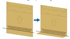
**step 3** Position the mounting template on the floor, and mark the hole positions on the wall according to the mounting holes indicated on the template.
