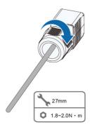
step 7 Pull gently backward the cable to ensure the connection is secure.
